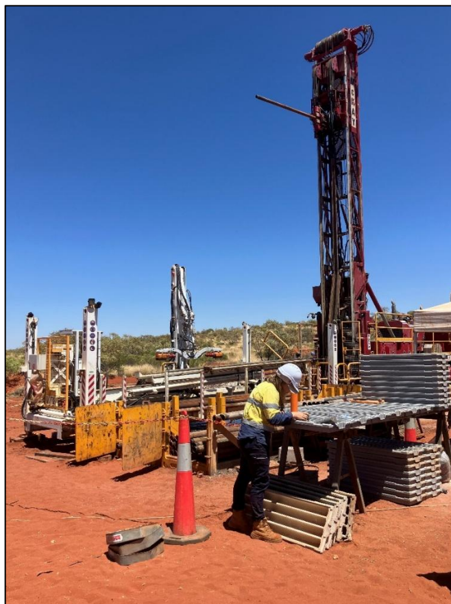
Figure 2 Iceni team member logging core at the WCD001 drill site at the Welcome Creek Project.
