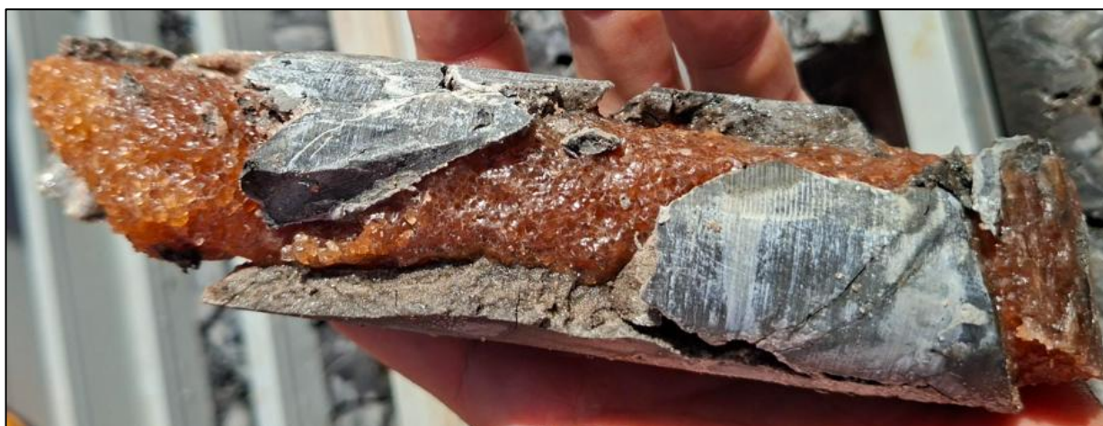
Figure 5 Example of brecciated zone from WCD001B at 1388.6m. The pink-orange coloured rock is halite (NaCl) or rock salt and represents approximately 50% of the core in this photo, The remaining grey coloured rock is mudstone. No sulphide mineralisation was observed in either rock.
