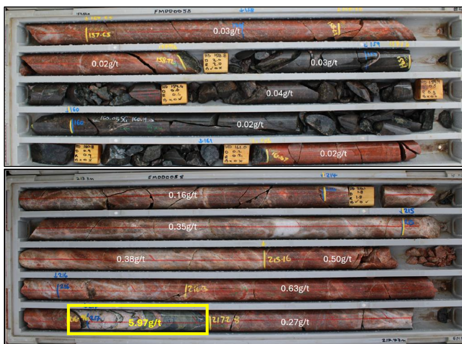
Figure 2 Core photos from FMDD0058 with gold grades (white): top, 157.52–161.36 m, unaltered lamprophyre (158.8–161.0 m); bottom, 213.3–217.73 m, silica-carbonate altered and sheared quartz syenite intruded by lamprophyre (216.96–217.20 m), bounded by high-grade quartz veins (yellow box see below Figure 3) (ICL ASX 1 September 2026)
