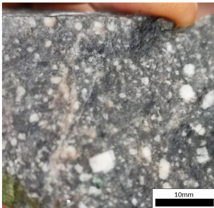
**Figure 12:** FMDD0047 Altered felsic porphyry with fine disseminated pyrite throughout.
