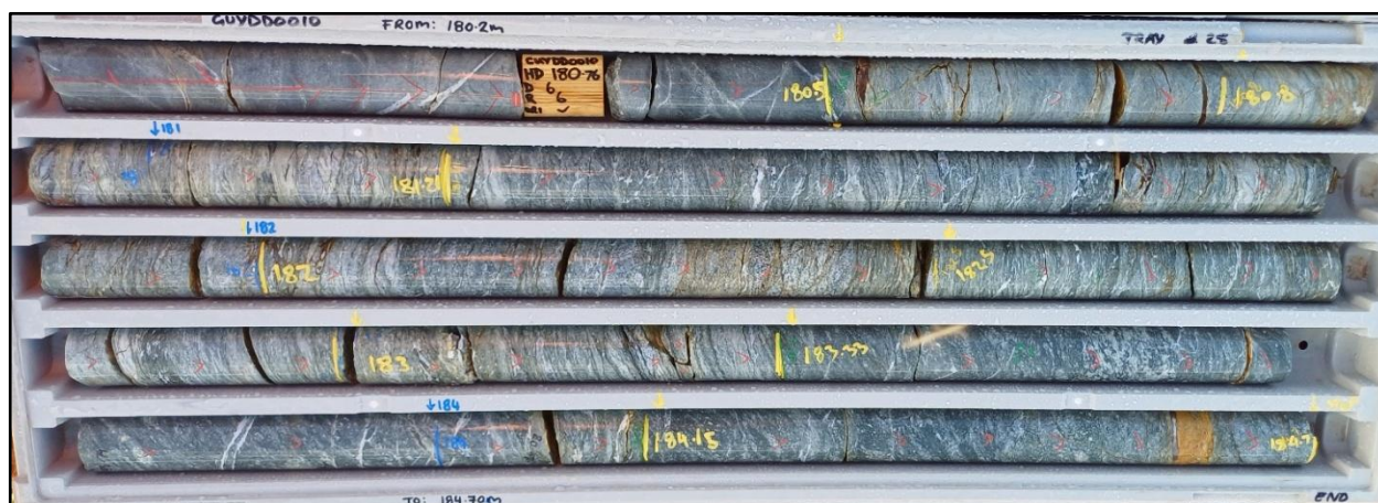
Figure 9 GUYDD0010 core tray photo 180.20m – 184.70m showing the intersected strongly sheared and sericite-chlorite altered volcaniclastics of Welcome Well Formation interpreted to be distal to the mineralised structure.
