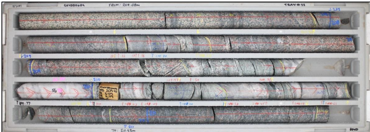
Figure 5 GUYDD0009 core tray photo 207.08m – 211.53m intercepting narrow mineralised shears which returned significant intercept of 8.59m @ 0.47g/t Au from 207.94m incl. 0.24m @ 2.55g/t Au from 208.31m & 0.27m @ 2.35g/t Au from 209.73m.
