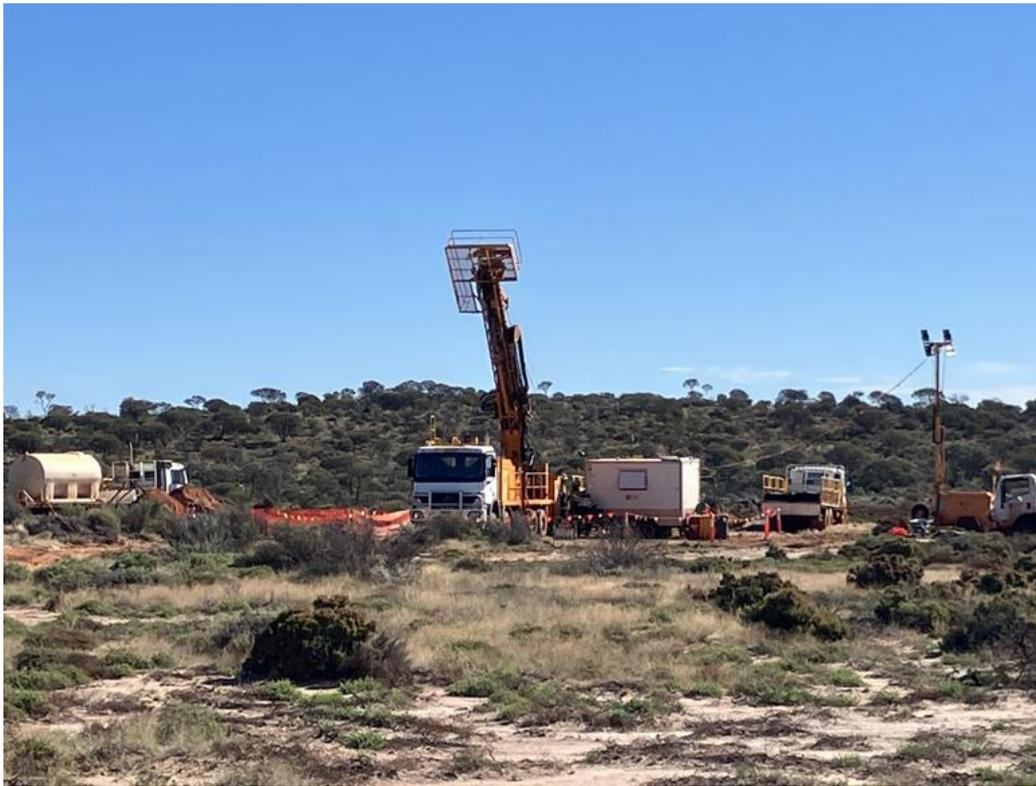
**Figure 9** Diamond drill rig operating on hole GUYDD0005, drilling west toward the Guyer Ridge in the background.
