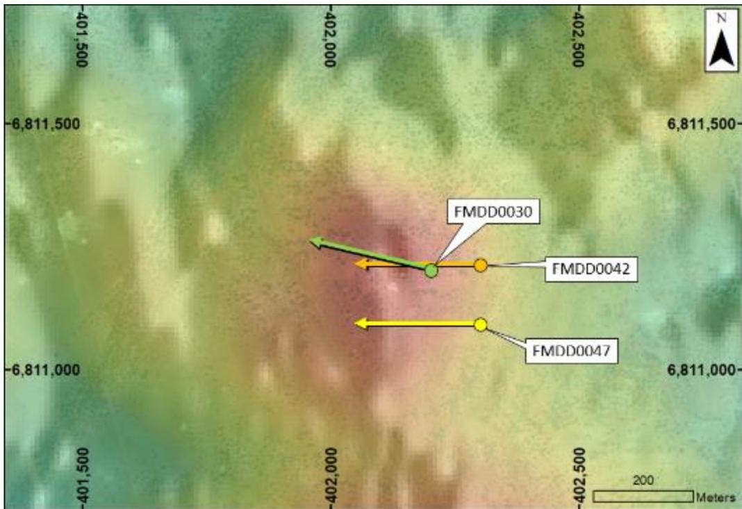
Figure 9: Collar plan showing the recent drilling at the **Recon 1** magnetic anomaly.
