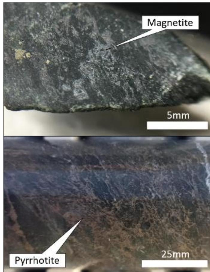
**Figure 11:** The magnetic response was caused by appreciable concentrations of the alteration minerals pyrrhotite and magnetite. The upper image is of drill core with abundant steel grey-coloured magnetite, example from ~390m in FMDD0042. The lower image is of drill core with abundant brown coloured pyrrhotite, example from ~473m in FMDD0042.
