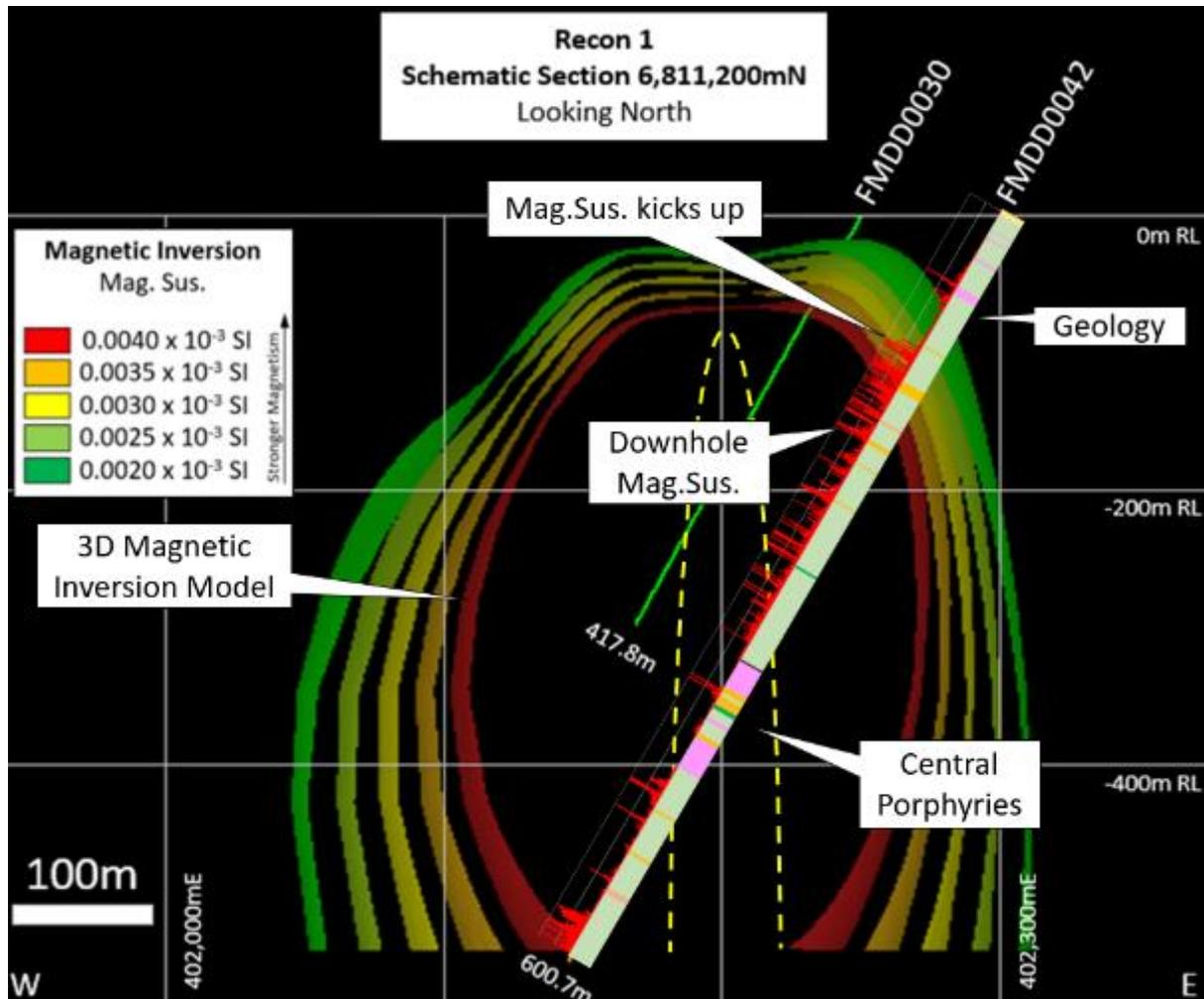
**Figure 2:** Schematic section 6,811,200mN showing the 3D magnetic inversion model intersected by FMDD0042. The DD has downhole geology and corresponding Mag Sus readings to demonstrate the strong magnetic halo that has developed surrounding the central intrusive porphyries. The Mag Sus shows a marked kick up as the DD enters the modelled magnetic body. It is interpreted that the porphyries are the engine that drove the development of the magnetic shell and the associated mineralisation.
