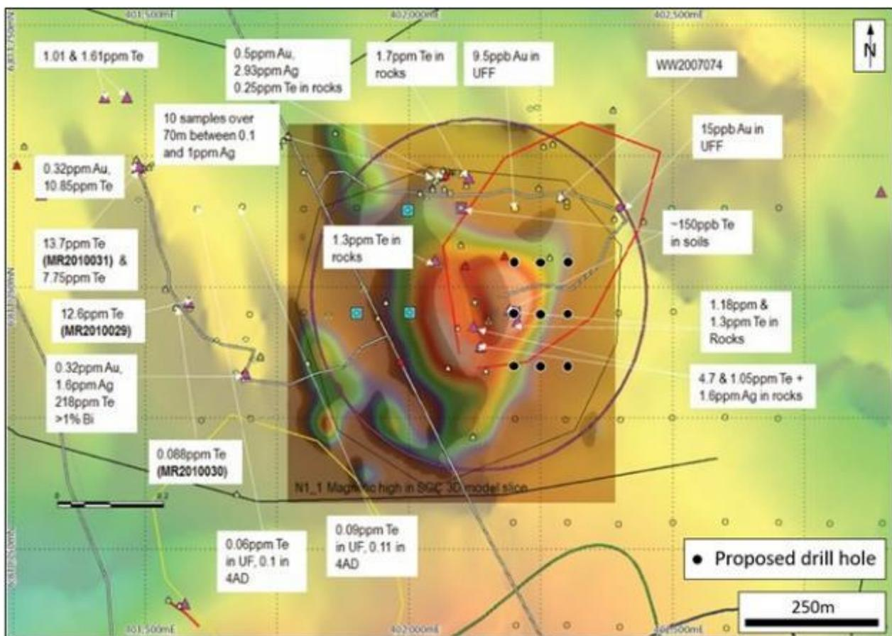
**Figure 6:** Surface rock chip results at **North 1** are anomalous in Ba/V, Au, Ag, Te and Bi. This geochemical association suggests a potential syenite intrusion at depth is the source.
