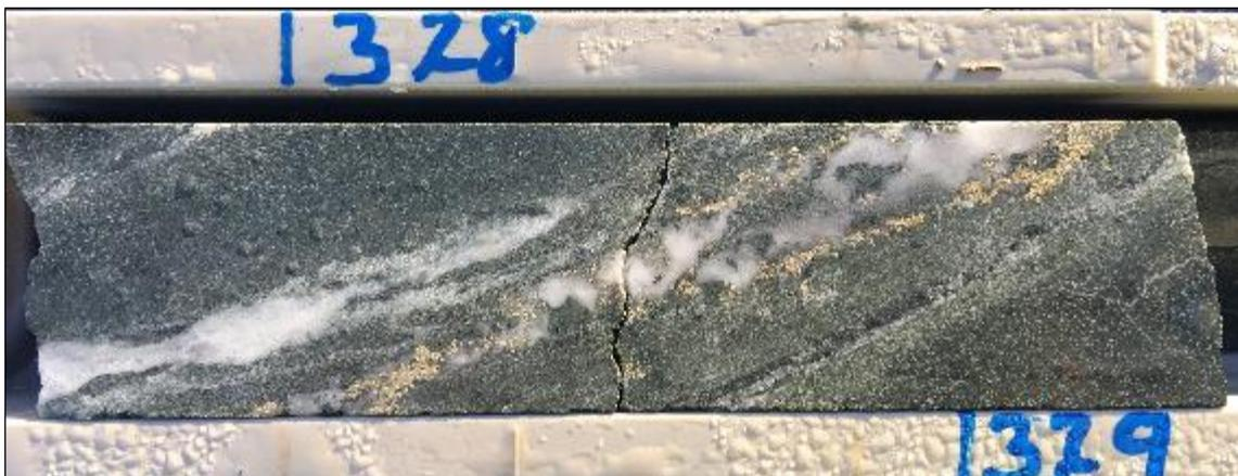
**Figure 3:** FMDD0042 ~328m, sulphide bearing quartz carbonate vein with pyrite. The alteration selvage is carbonate and magnetite altered andesite.
