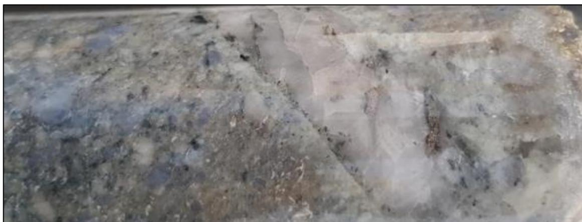
**Figure 14:** FMDD0042 ~66m Arsenopyrite and pyrite bearing quartz vein within altered felsic porphyry.
