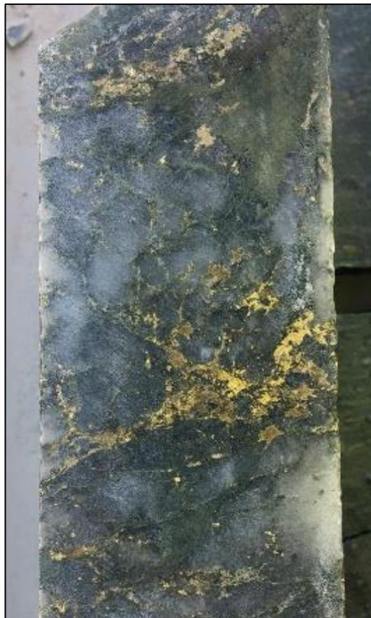
**Figure 1:** FMDD0042 ~135m, sulphide bearing quartz vein with pyrrhotite, pyrite and chalcopyrite hosted within altered andesite volcanics.
