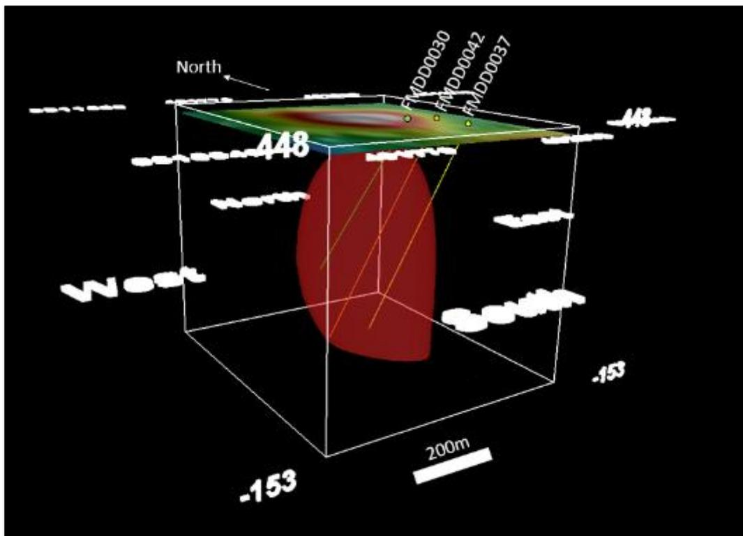
Figure 10: Orthographic view of the **Recon 1** magnetic anomaly and magnetic inversion model showing DD holes FMDD0030, 42 and 47 piercing the modelled magnetic body.
