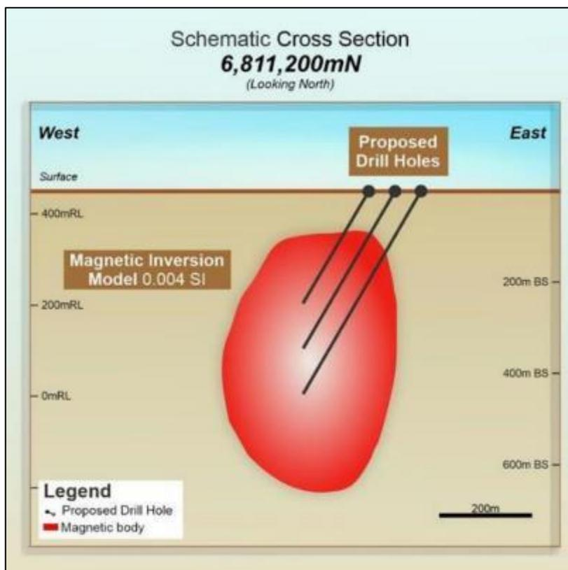
**Figure 8:** Schematic section 6,811,200mN through the **Recon 1** magnetic inversion model.
