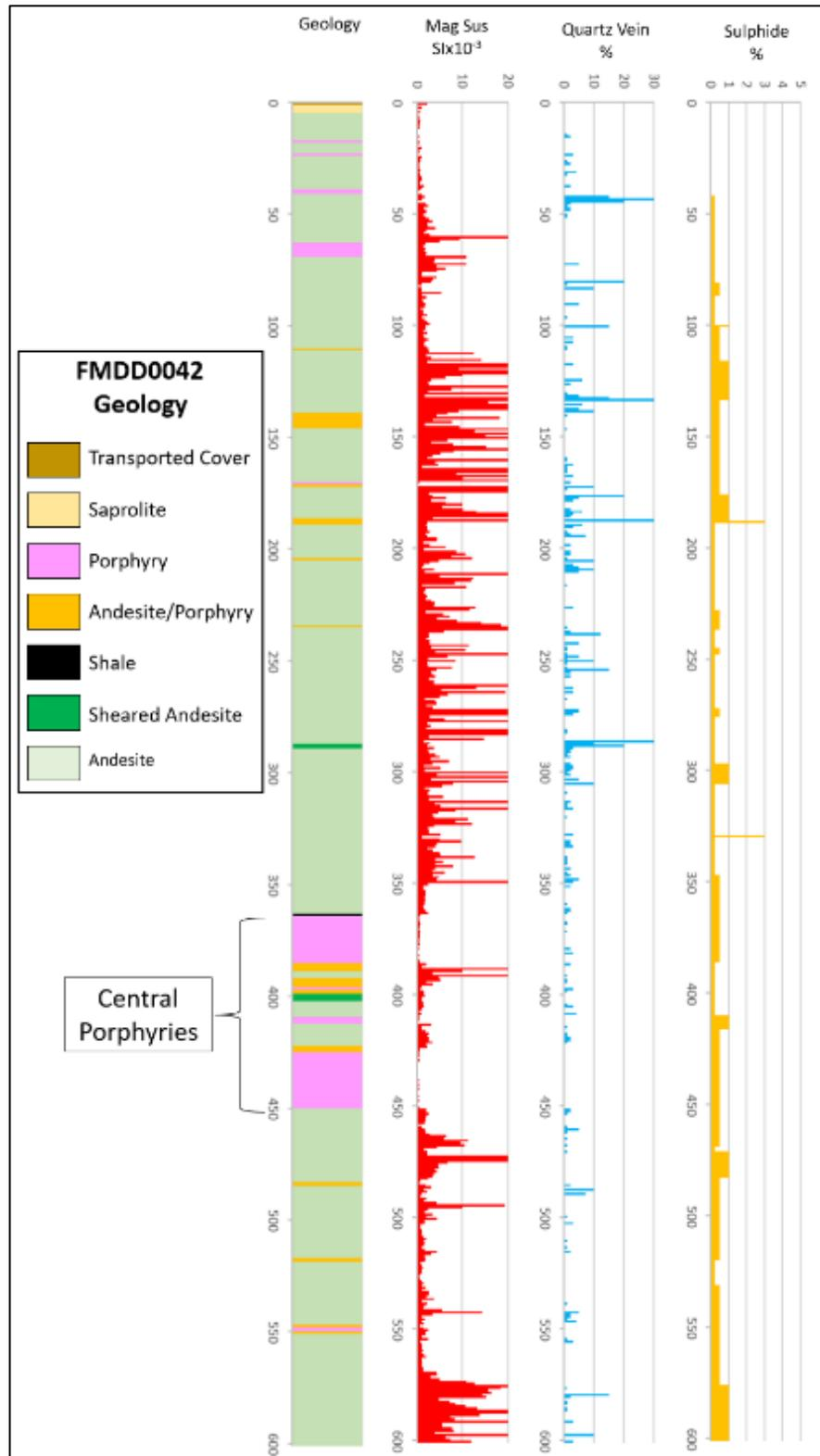
**Figure 12:** FMDD0042 correlated downhole logs for geology, Mag Sus, quartz veining and sulphides. The Mag Sus demonstrates there is a magnetic halo surrounding the central porphyry intrusions. There is a strong association between increased magnetism, increased quartz veining and increased sulphides within hole.
