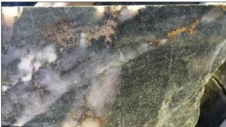
**Figure 13:** FMDD0042 ~135m, sulphide bearing quartz vein with pyrrhotite, pyrite and chalcopyrite hosted within altered andesite volcanics.
