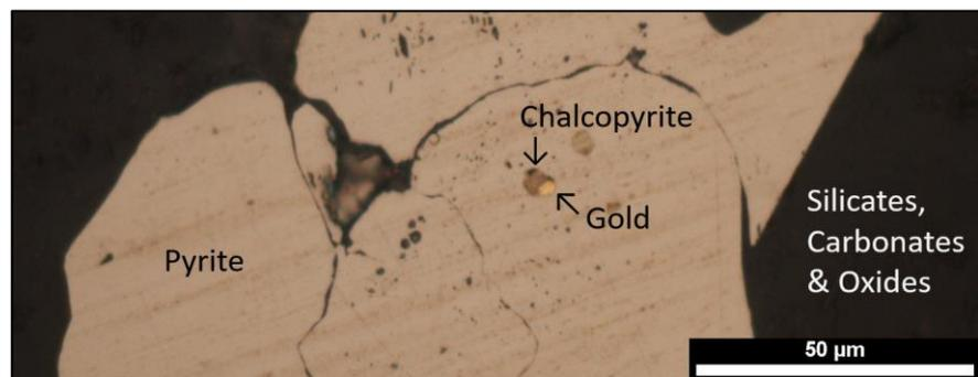
**Figure 1:** Photomicrograph of gold at 224.6m in drill hole FMDD0032.
