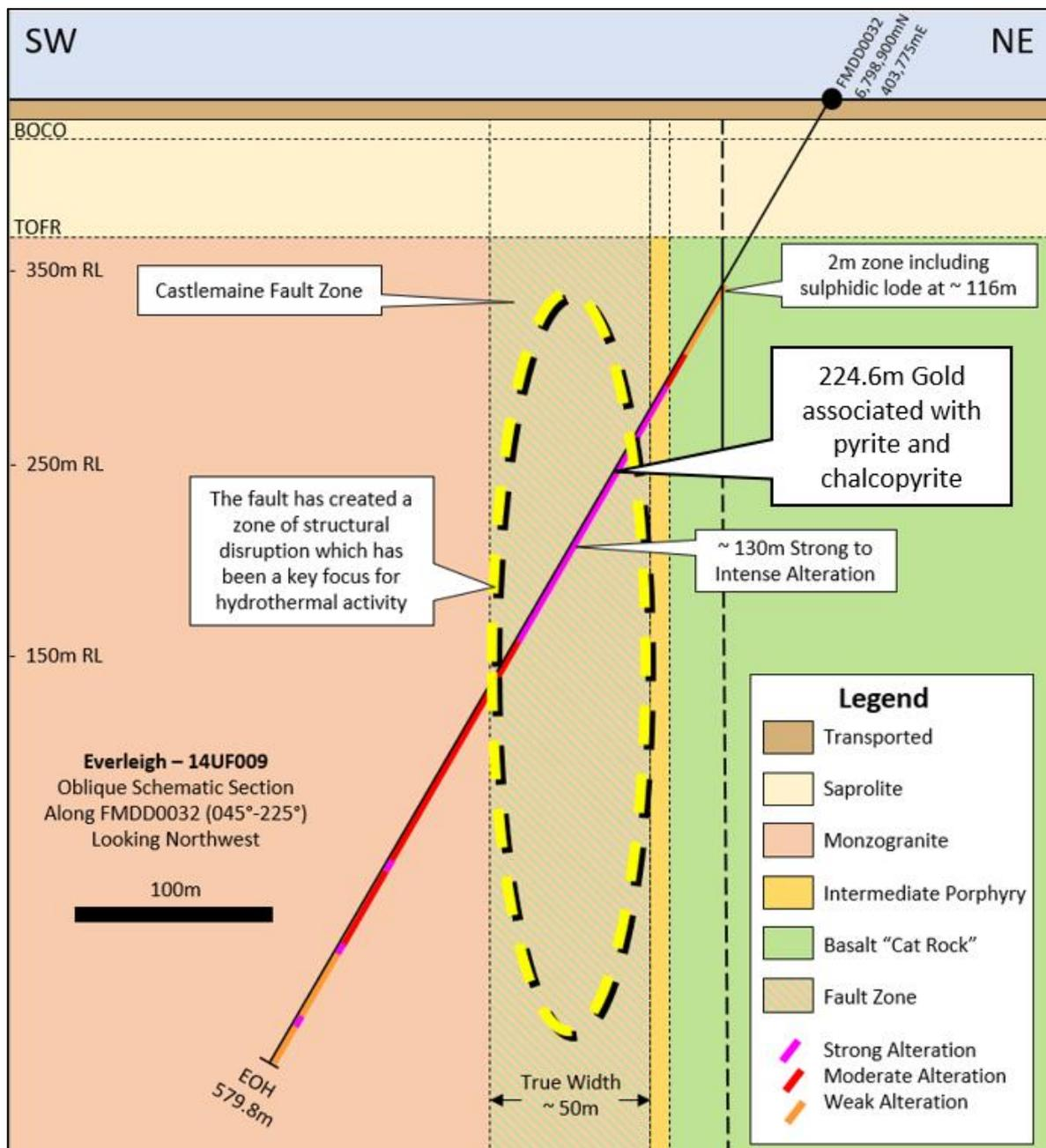
**Figure 2:** Oblique schematic section along **FMDD0032** through the Castlemaine Fault. **Gold** was identified at a depth of 224.6m, within the **~130m thick zone** of strong alteration within **FMDD0032** through the Castlemaine Fault.
