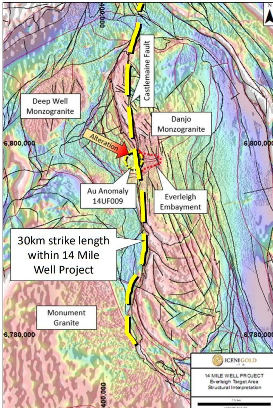
**Figure 6:** Approximately 30km strike length of the prospective **Castlemaine Fault** is located within the 14 Mile Well project. To the south the fault is spatially associated with known gold mineralisation at Yundamindera. To the north the fault interacts with the **Celia Fault Zone** within the **Claypan Target** area.
