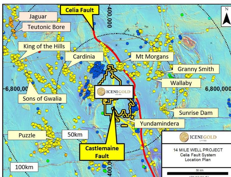
**Figure 5:** The **Celia Fault** zone passes along the eastern margin of the 14 Mile Well Project while a fault splay, the **Castlemaine Fault**, passes through the centre of the project. Drillhole **FMDD0032** was designed to test the **Castlemaine Fault** in the **Everleigh** target area.
